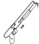
The shells are stored in a tube under the barrel, so the weapon cannot accept underbarrel mounts. The sling attaches to the end of the magazine and to the rear of the weapon on its right, just under the ejection port. It does not have a stock for ease of use.
